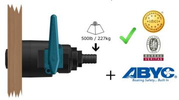
TRUDESIGN™ Skin Fittings (Thru Hulls), when assembled together with TRUDESIGN™ Ball Valves and Load Bearing Collars, comply with ABYC H-27 standards. This allows the entire assembly to withstand a 500lb (226.8kg) load applied to the inboard end of the assembly (i.e. from the Ball Valve's Tail fitting) for a minimum of 30 seconds without any damage occurring.
