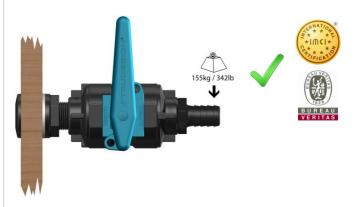
In accordance with ISO 9093-2 standards, Skin Fittings (Thru Hulls) are subjected to a 155kg (341.7lb) load, applied to the threaded section for a minimum of 30 seconds, without any damage occurring.
